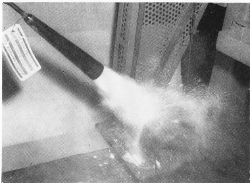
A five-pound Carbon Dioxide extinguisher makes short work of putting out a possible fire in a small motor. As pictured, the extinguisher nozzle should be held down close to the motor. Of course, the electrical plug was first removed from the wall socket so that the source of power was cut off.
